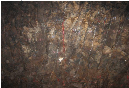
Fig.5 The Appearance of upper segment of weak weathering of Columnar Jointed Basalt(the 68 th adit in Baihetan dam site)
