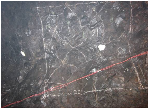
Fig.3 The Appearance of slightly weathering of Columnar Jointed Basalt (the 36th adit in Baihetan dam site)
