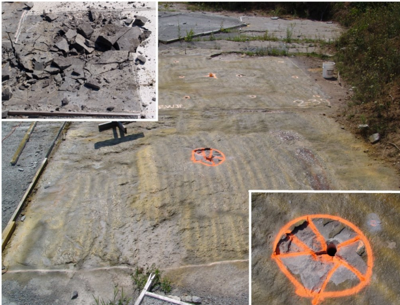
Figure 3. Blast damage to unsupported and RockWeb supported rock
