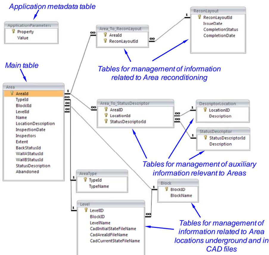
Figure 2. Diagram showing the MS Access database tables and the general structure used to manage the audit data.
