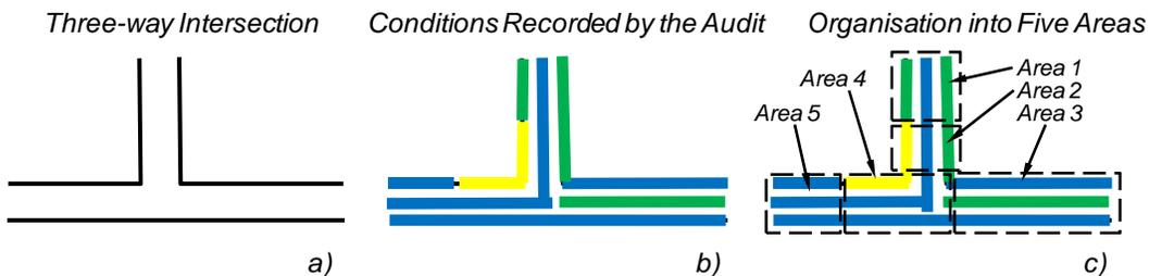
Figure 1. The concept of *Area* is illustrated using an example in a three-way intersection (a). The audit established ground support condition categories in accordance with the guidelines (b). The audited section is subdivided into *Areas* (c). In each *Area*, the audited condition in either wall or back remains constant.
