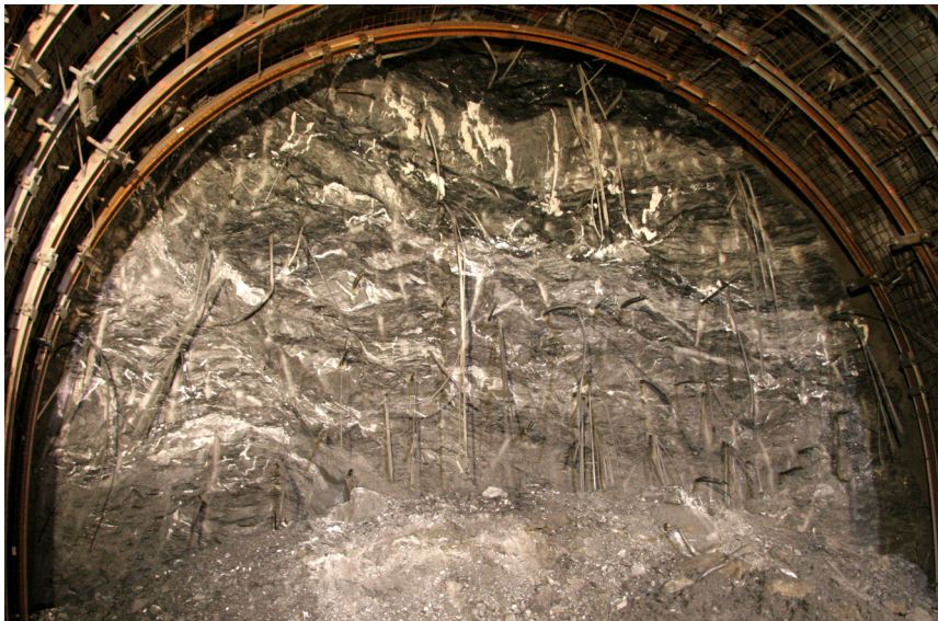
Figure 2. Example of appearance of the graphitic schists of Houiller at the tunnel face.
