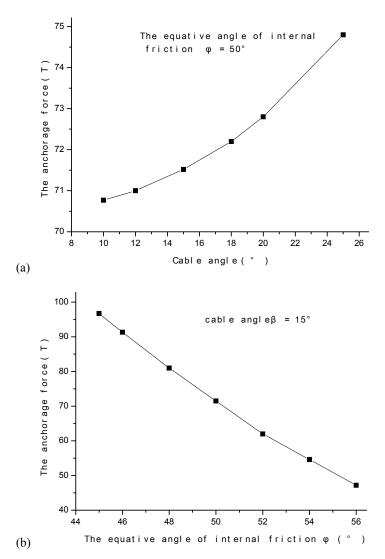
Figure 3. Relationships between: a) anchor force and cable angle; and b) anchor force and friction angle.
