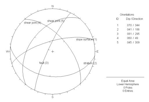
Figure 2. Main joints relative to slope surface for the case study.
