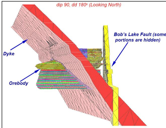
Figure 3. Looking north at 153 Orebody, diabase dyke and Bob's Lake Fault (Mortazavi et al 2000)
