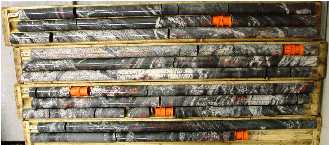
Figure 8. Condition and drill recovery for the OD4984 oriented core at approximately 2600m below surface .
