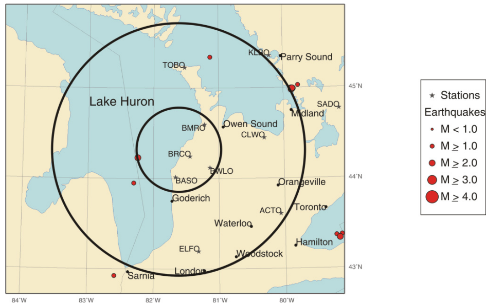
Figure 5: Micro-seismic Borehole Seismometer Network (BASO; BMRO; BWLO) within 50 km of Bruce site and Micro-seismic Monitoring Data Reported for 2007.
