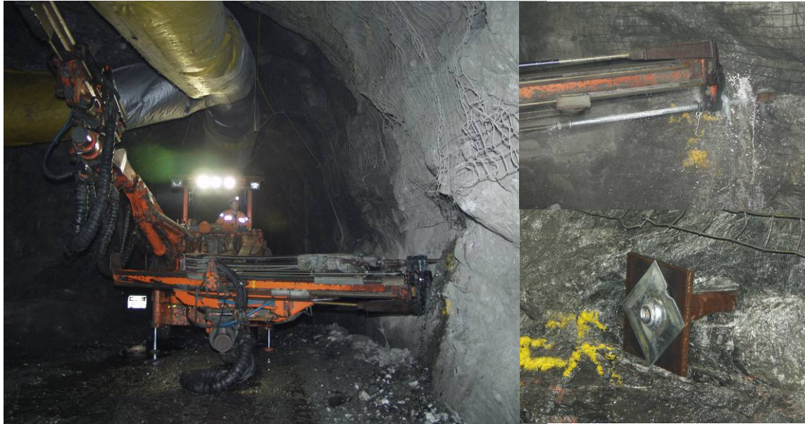
Figure 8. Installation of a split tube bolt into a rough simulated borehole.
