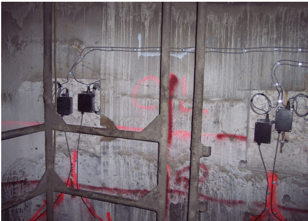
Figure 5. Photograph showing the four surface-mounted extensometers installed in the #3 Shaft. Extensometer enclosures are recessed inside the shaft wall to allow for unobstructed movement of the cage.
