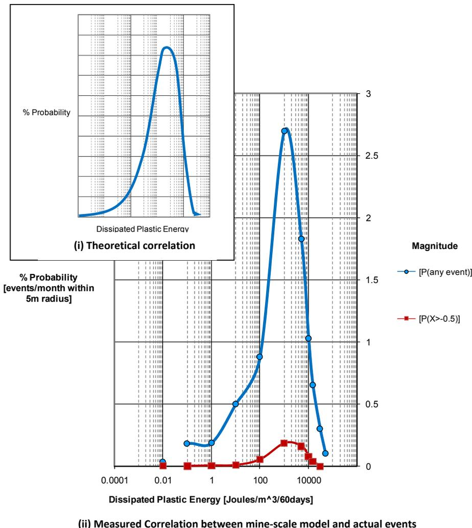
Figure 6 Correlation between DPE and event probability from a mine-scale analysis at an example mine
