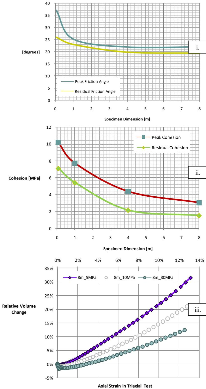
Figure 3. Relation between (i. and ii.) specimen dimension and selected material properties and (iii.) volume change, axial strain and confining pressure for a selected specimen
