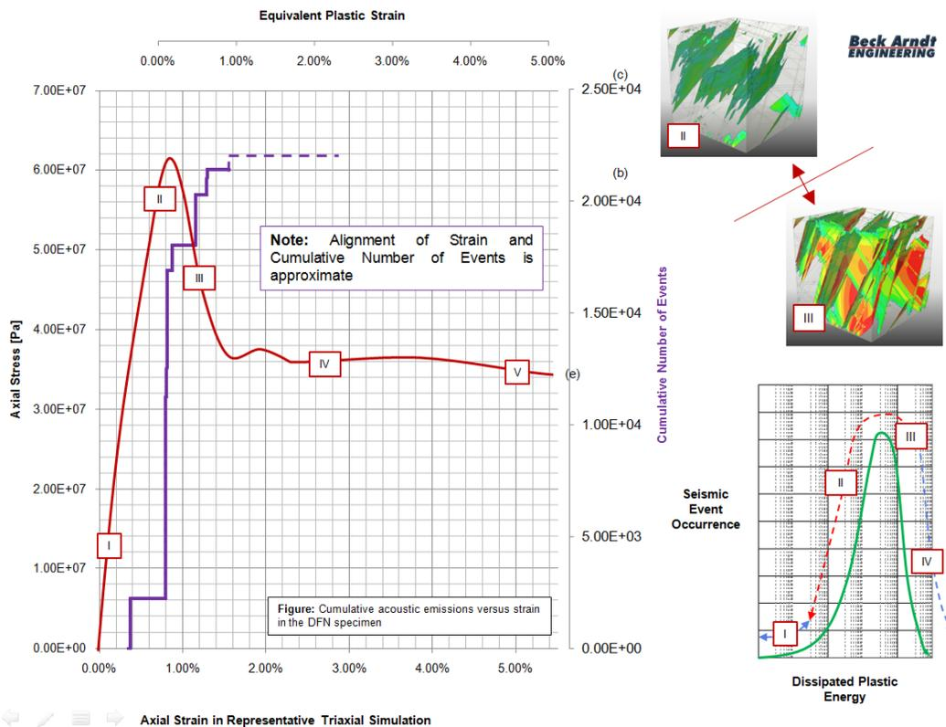
Figure 5 Correlation between stages of deformation and acoustic emissions for a DFN specimen
