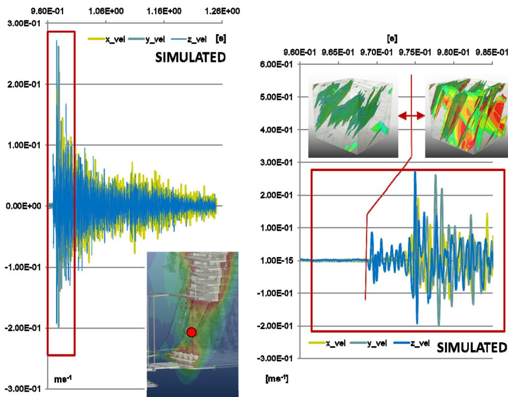
Figure 7 Simulated Seismogram of event occurring at transition from Phase 2 to 3. “Measured” at a corner node of the DFN sub model, loaded using stress path at the point shown in the block cave global model.
