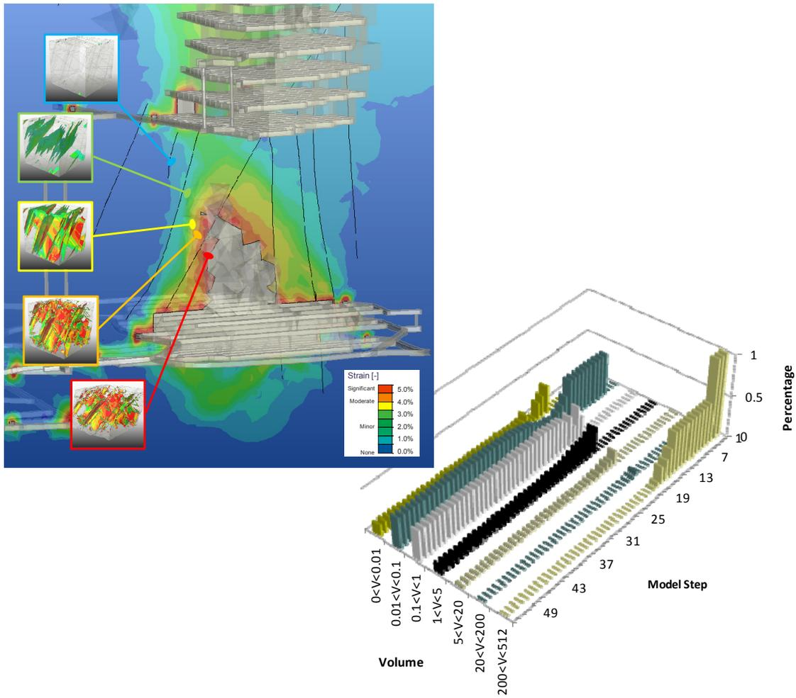
Figure 8. Changes to the P80 size fraction at selected locations above the undercut, forecast using DFN Abaqus models
