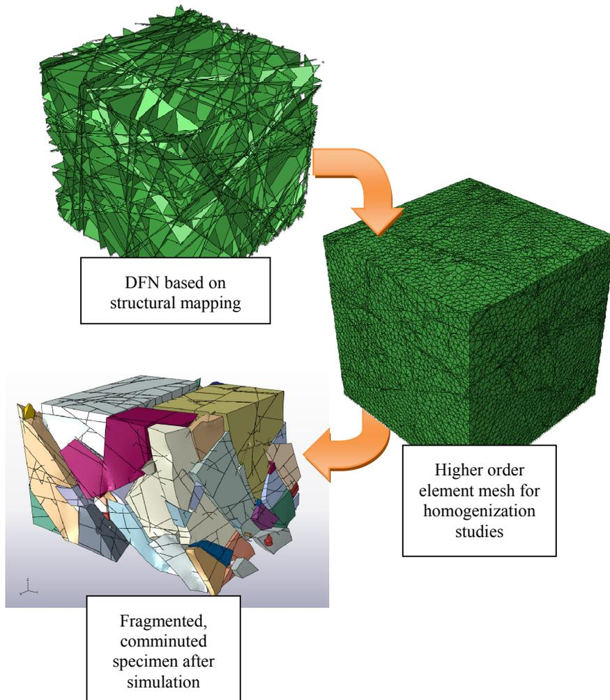
Figure 1. An example of a DFN model of skarn
