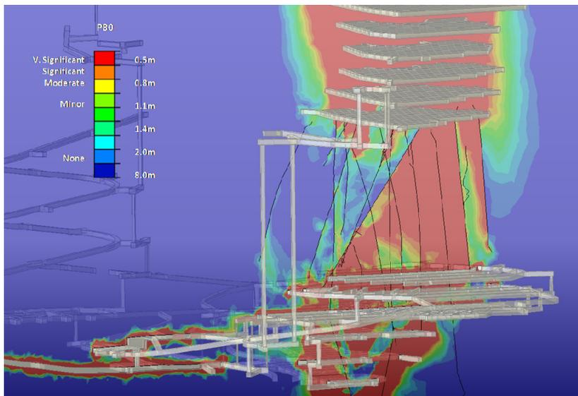
Figure 9. P80 (size of the 80<sup>th</sup> percentile fragment) on a section through an entire cave column. Any size fraction can be plotted
