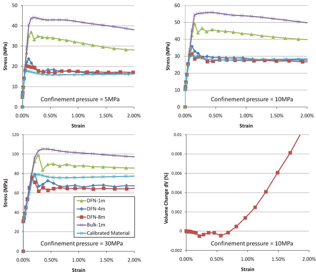
Figure 2. Stress-strain response of DFN representations of differing volumes of a rock mass subjected to three different states of lateral confinement
