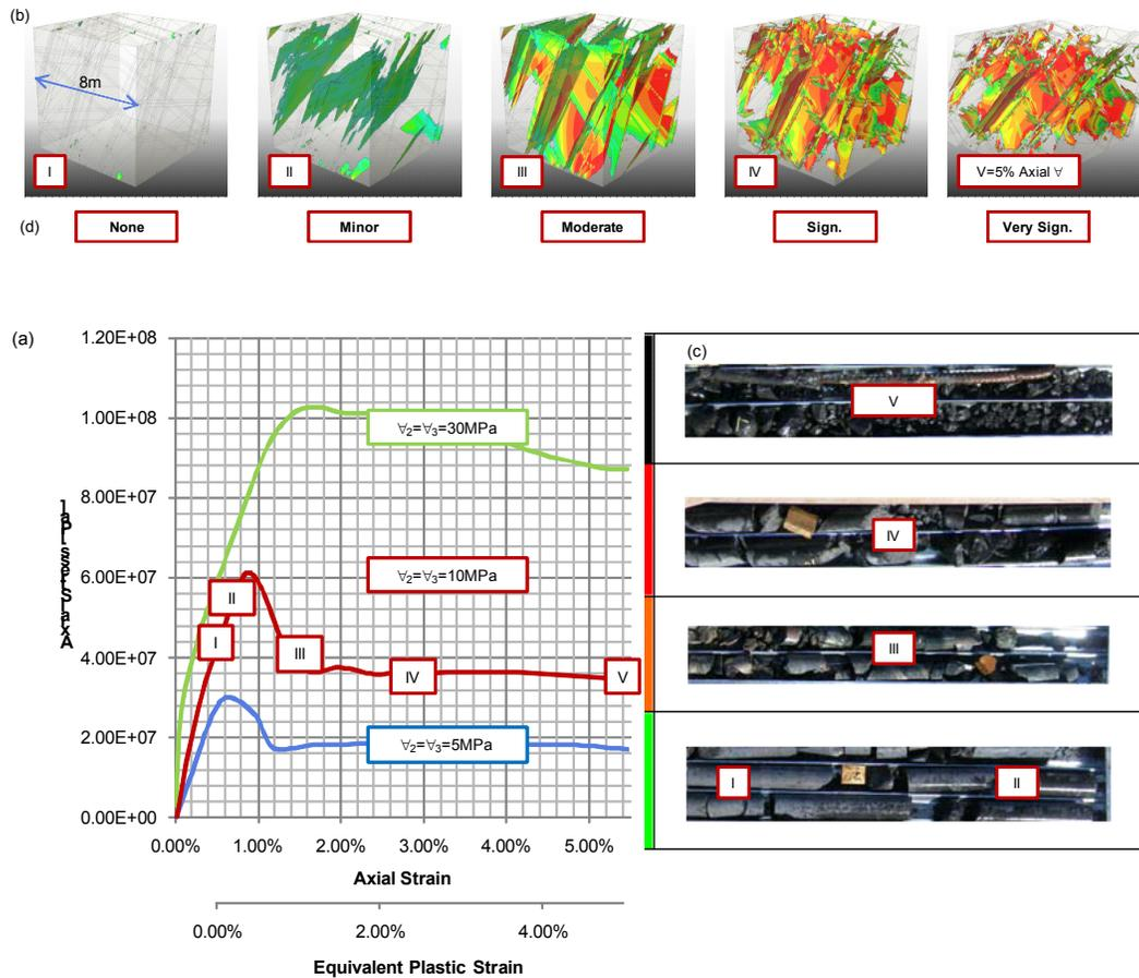
Figure 4. Comparison of (a) Stress-strain response of a simulated rock mass specimen (8m diameter) at varying levels of confinement. (b) The yield state of discontinuities and the deformation of the specimen at milestones of yield (c) photographs of diamond drill core specimens, simulated by the global model to be at these respective states of strain (d) the Common Damage Scale.
