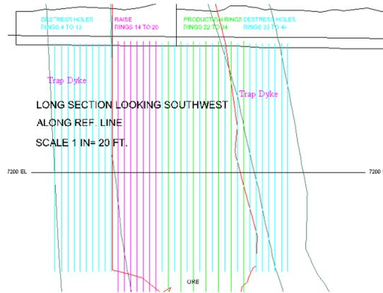
Figure 8b: Section showing de-stress holes laid out in trap dykes and the 9281stope (3710-3880 L).
